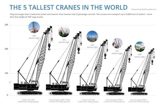
The crawler-type crane Liebherr LR 13000 exceeds the world's highest church tower – the Ulm Cathedral (162m) – by as much as 86 metres. This makes it the world's largest mobile crane. Inconceivable: By combining the 120 m long main mast with the 126m long luffing jib, the monstrous lattice mast system achieves an impressive 246 m.
